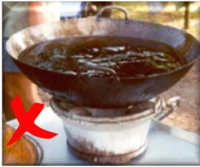
Figure 26. This wok is too full of oil, the burner is not certified, and the burner is not secured, the wok is unstable. This is not suitable at an event.
