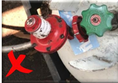
Figure 37. This is a high-pressure regulator; this is not suitable for use at an event.
