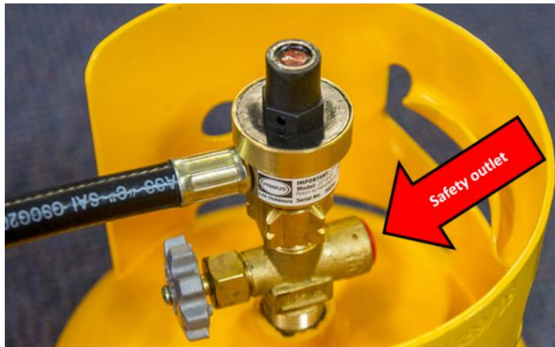
Figure 9. Gas bottle safety pressure valve
