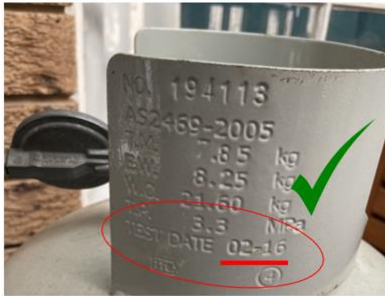
Figure 6. Example of compliant gas bottle that has been tested within the last 10 years this was tested in 2016 and is ok until 2026.
