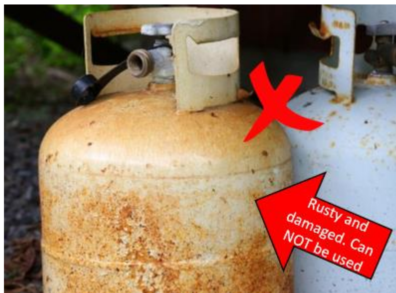
Figure 5. Rusty, damaged gas bottle. This would not be allowed on site
