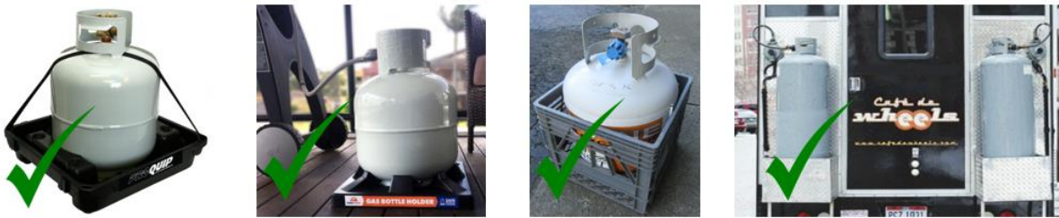
Figure 7. Examples of suitable gas bottle storage
