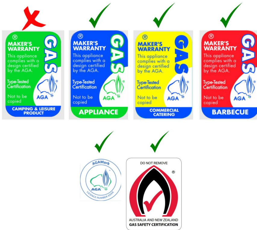
Figure 4. Some examples of approved gas certification labels
