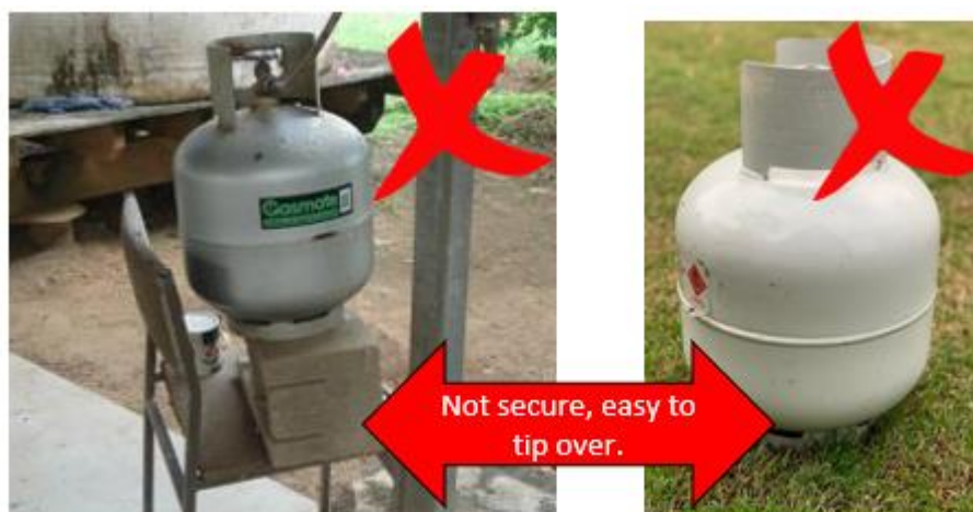
Figure 8. Examples of unsuitable gas bottle storage. This would not be allowed on site
