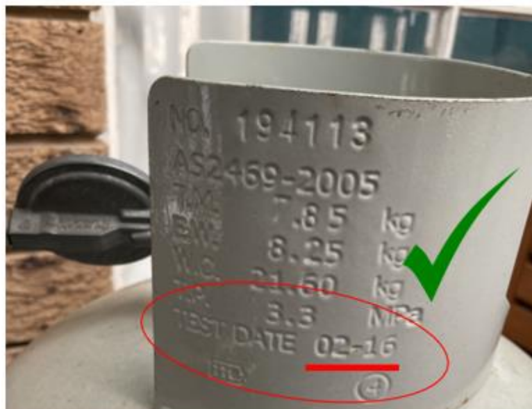
Figure 6. Example of compliant gas bottle that has been tested within the last 10 years.
