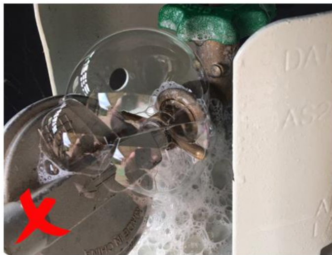
Figure 10. Image shows soapy water test with bubbles = gas leak present, this must be fixed before this gas bottle can be used.
