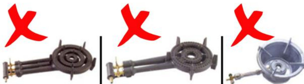
Figure 25. These gas rings do not have a certification label (as per figure 3.), they are not able to be secured to the bench and pots can easily tip when sitting on these burners. These are not suitable for use at events.
