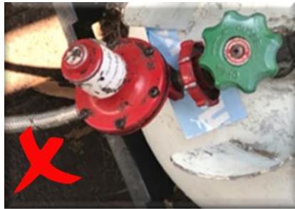
Figure 47. This is a high-pressure regulator; this is not suitable for use at an event.
